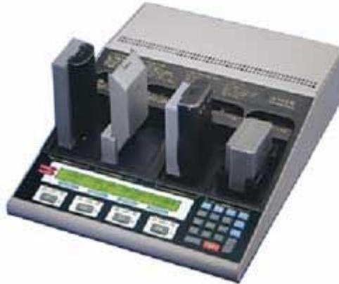
**Figure 4.** The Cadex C7000 battery analyzer measures internal battery resistance. The milliohm readings can be read as part of a quick-battery test or can be included in the recondition program.
